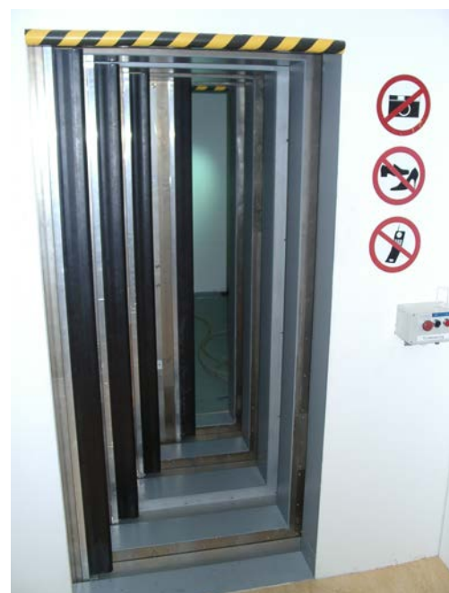
The picture shows the entrance to the magnetically shielded room at PTB Berlin.
