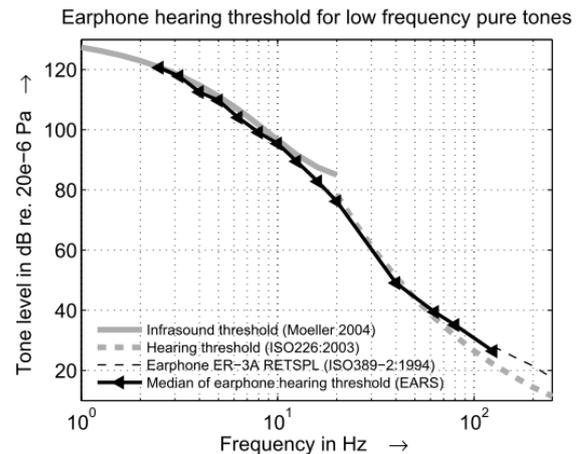
Determined hearing threshold from 125 Hz down to 2.5 Hz (black line). The gray lines show the free field threshold (broken line) and the estimated threshold for infrasound frequencies from literature [1] (solid line).
