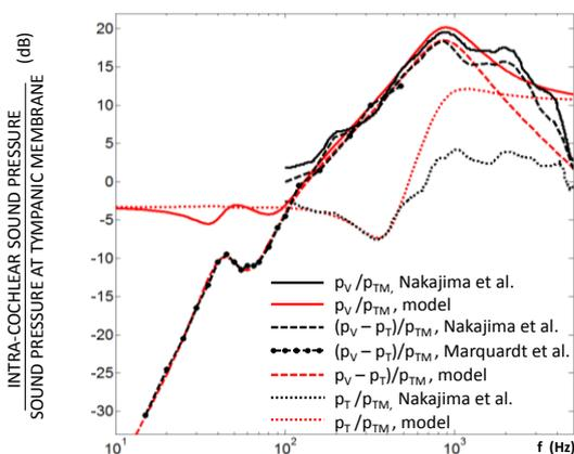
Measured and simulated sound pressures in the inner ear relative to the ear canal (see page 2).
