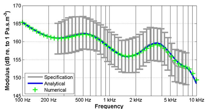
Modulus (in dB re. to 1 Pa.s. m<sup>-3</sup>) versus frequency of the acoustic input impedance of the ear simulator for the neonates group. Gray curve: Specifications and standard deviation. Blue curve: Analytical model. Green crosses: Finite element model.
