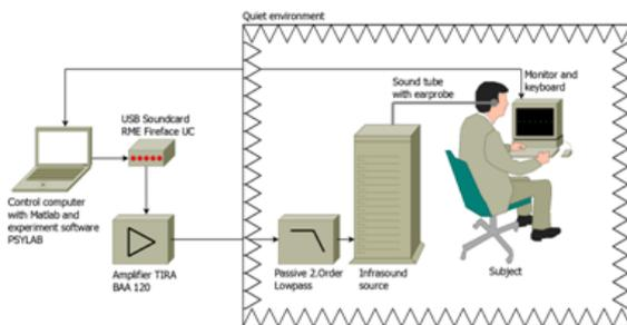
Setup for the measurement of the insert earphone hearing threshold for low and infrasound frequencies
