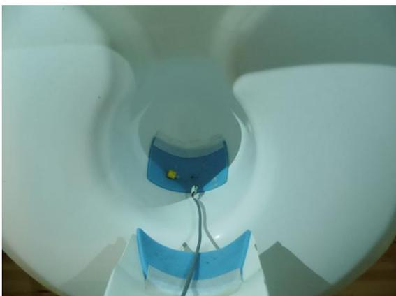
MEMS transducer under evaluation for compatibility for use within the MEG test facility
