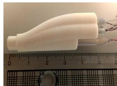
The picture above shows the final transducer assembly, which is intended to be coupled to a human ear via a foam ear plug around the 5 mm diameter acoustic output port. Initial measurements showed that with a conservative drive level, the SPL exceeded 90 dB between 60-70 kHz. The target of over 100 dB is considered easily achievable with an increased drive level.
