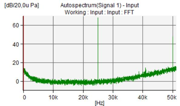
SPL of MEMS transmitter driven with 1.77 V at 25 kHz. Peaks at 25 kHz and 50 kHz can be seen.
