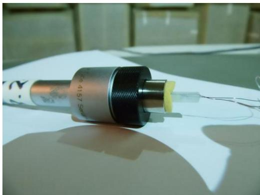
MEMS transmitter inserted in Brüel & Kjaer type 4157 occluded ear simulator.
