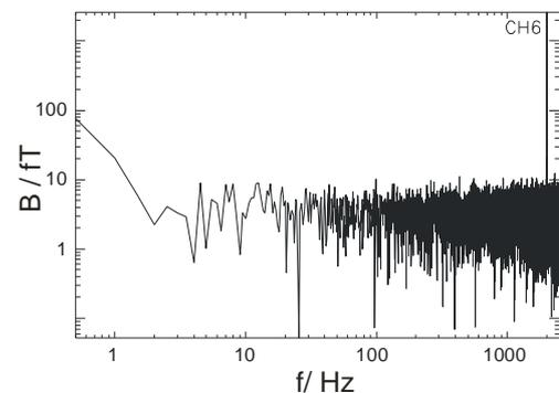
Power spectrum of a MEG channel in the vicinity of the transmitter running at 2 kHz (note the line in the response at 2 kHz)
