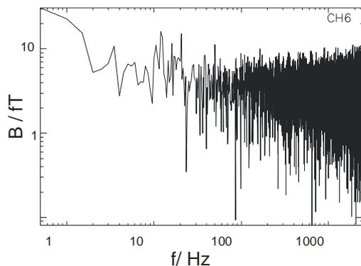
Power spectrum of the same MEG channel, but for the transmitter at 25 kHz (note the different y-axis scaling)
