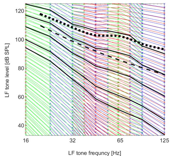
Figure 5: ELCs (thin black; 10, 20, 40 60 & 80 phon) were derived from a loudness gradient field (colored lines; average data from 12 subjects). ELCs (40 - 80 phon) show a similar step as the average METF (dotted). ISO 226:2003 does not show such step (dashed; 60-phon isophon).
