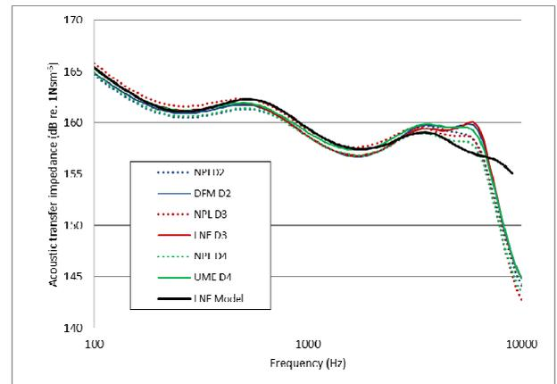
Figure 3: Results from the round-robin calibration exercise to validate the acoustic transfer impedance characteristic of the neonatal occluded ear simulator. Note that typical measurement uncertainty in each curve is around 0.5 dB.
