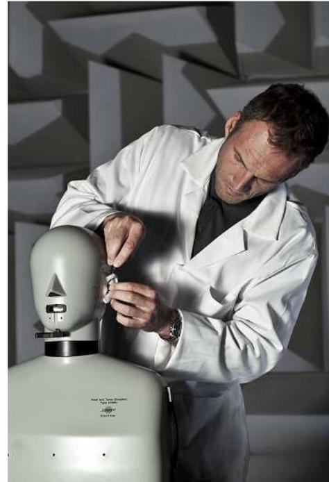
Figure 8: Acoustic testing on a Brüel & Kjær Head-And-Torso Simulator.
