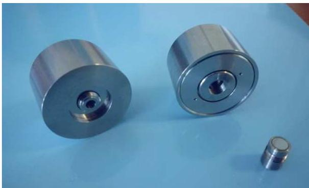
Figure 1: Prototype ear simulators for neonatal hearing assessment designed against a specification derived from clinical and anatomical data.
