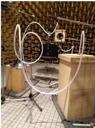
Measurement setup for hearing threshold measurements for infrasound combined with audiosound.
