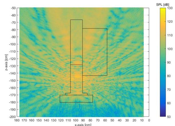
Sound field in front of the welding machine as measured in laboratory reference workplace setup
