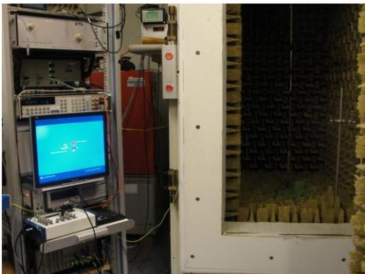
Novel primary calibration setup for quarter inch microphones up to 150 kHz.
