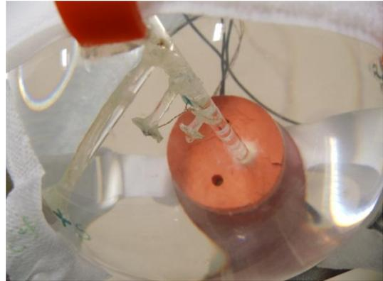
View into the fluid filled sphere filled with electrode pairs.
