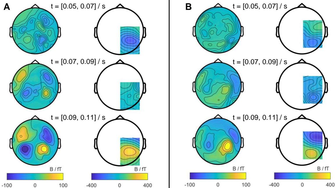
Magnetic field distribution maps for two subjects (A and B) obtained with SQUID-MEG (left column in each picture) and OPM-MEG (right column)
