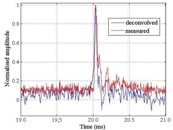
Microphone output signal and result following deconvolution of the microphone transient response
