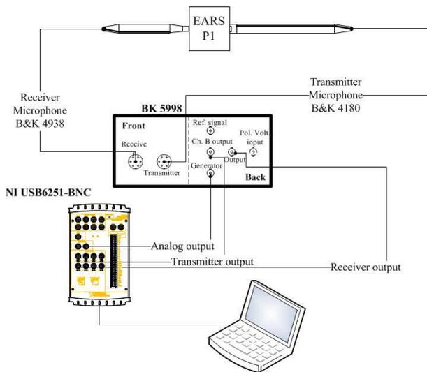
Schematic representation of the set-up for measuring the transient response of the ear simulator
